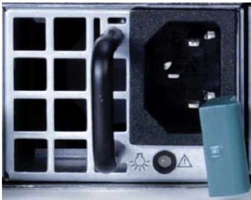
Figure 18. Removing a PSU from the chassis
